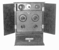
**GECOPHONE BC 2001 -** This is a two-valve receiver manufactured in Great Britain in 1922, with bottom compartment for battery storage. (*Greg Farmer - Fridley, MN*)
