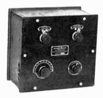
Figure 12. 2B tuning unit, panel view.
