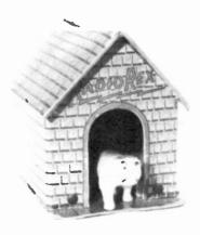
RADIO REX - This very unique piece was manufactured in 1922 by the Elmwood Button Company in Stratford, Ct. The house is composed of heavy cardboard, and the dog is made of celluloid with the consistency of a ping-pong ball. The dog is held in by a solenoid magnet, but rushes out when you call or clap your hands, due to the "imperfect contact" connector. (Walter V. Worth - Wollaston, MA)
