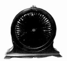
VICTOR LUMIERE #1 - This is one of a few speakers produced worldwide that utilizes a pleated paper diaphragm to produce sound. This feature supposedly made the speaker more omni-directional. (Greg Farmer - Fridley, MN)
