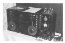
An SE-143 (IP-500) receiver, SE-1071 1-tube detector and SE-183A triple-crystal detector. (Tom Pamula)
