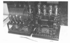
RCA ET-3619 Transmitter and ET-3620 Kenotron Rectifier. Four UV-202 tubes give 20-watts CW cutput between 180 and 320 meters. 10-watts is obtained on phone. UV-216 Kenotron rectifier tubes are used in the ET-3620. (Nevell Greenough)
