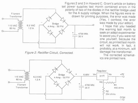
Figure 3. Complete "A" Voltage Schematic, Corrected.
