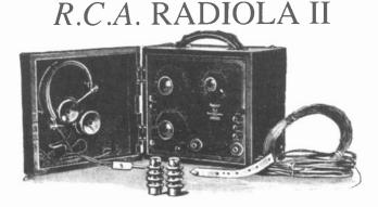
This is an exceptionally high class receiving set designed particularly for use where portability is desired. Light in weight yet ruggedly built into a convenient carrying case with special compartments to accommodate the headset, two tubular three-cell flash light "A" batteries and from two to four "B" batteries. The batteries are at all times connected allowing instant operation by only connecting an antenna and ground.
