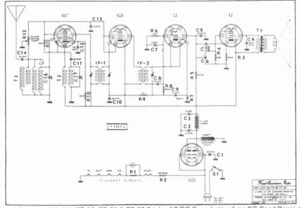
Freed-Eisemann Models FE-52, FE-56 & FE-58 5-tube AC/DC Superheterodyne BC Band Receiver.
