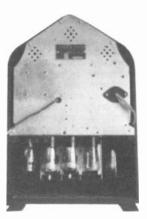
GLORITONE MODEL 27 – Two views of an unusual cathedral made in 1930 by U. S. Radio and Television Corp. Note that the chassis is mounted upside-down. It uses a 27, a 45, 2-24's, and an 80. (Alexandria Nelson -Albuquerque, NM)
