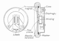
Figure 3. The internal construction of a headset (Reyner, Modern Radio Communication, 1923).
