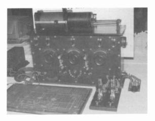
The Best-of-Show winning contest entry on the left is an early receiver with buzzer transmitting circuit from 1908 made by the radio and aviation pioneer, Elmo N. Pickerill (Dr. R. Muchow). Below left is an Adams Morgan Paragon Model Two introduced in late 1924. This was the two-tube model in a lineup which included the three-and four-tube Models Three and Four (C. Mooney). Below is the Crosley Model RFL- 60, collectible because of its gold-screened design on its pane.
