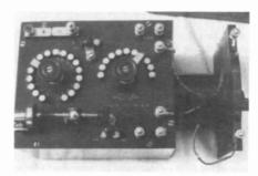
IP -111 - Made by Wireless Specialty Apparatus (WSA). This is the 1907 Navy version of the IP76 receiver, the first to utilize a loose coupler and also the first completely self-contained receiver. It is in its original case, with its original headphones. On the right is a close-up of the IP-111. (Jim Kreuzer - Alma, NY)
