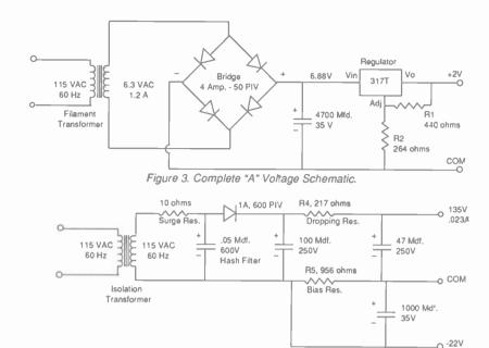
Figure 4. Complete "B" and "C" Supply Schematic.
