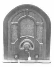
**BEL-RAD** - A six-tube superhet mantel radio of unknown manufacture. It uses a 47, 55, 57, 2-58's and an 80. The radio is quite cheaply made, but works well. I would appreciate any information on it. (*Frank Heathcote, Logansport, IN*)
