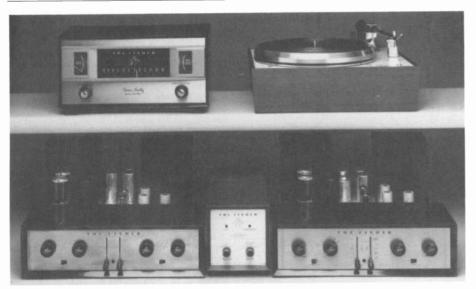
EARLY HI-FI - Top Shelf: Fisher FM 90X, 1957. The first of their famous "Gold Cascode" front ends, it also introduced the 6DJ8 tube to the U.S. market. Reko Kut Rondine 2 turntable (not affiliated with Fisher). Bottom Shelf: At center is an MPX 100 multiplex adapter (1962) flanked by a pair of 50C mono preamps driving a pair of 50A mono power amps (1952). (Stephen N. Raymer-Minneapolis, MN)
