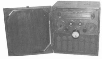
The RCA Radiola 26. The loop antenna is in the front cover on the left. The meter, usually missing, indicates filament voltage.
