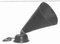
MEGAPHONE SPEAKER - This unmarked fiber horn speaker has a sheet metal base containing a Baldwin single phone in a clamp arrangement. (Wally Worth - Wollaston, MA)
