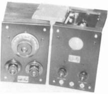
WESTINGHOUSE RT-AR-RA-DA - The two units on the right appeared in 1920 and are the commonly seen RA (shortwave regenerative receiver) and DA (detector and 2-stage amplifier). The RA and DA also were available in a single cabinet called the RC. The two units on the left appeared in 1922 and are seldom seen. They are the RT (antenna tuner) and AR (3-stage RF amplifier). Although these units were manufactured by Westinghouse, they were distributed by RCA. (C.A. Albion - Niagara Falls, NY)
