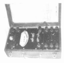
TEST INSTRUMENT - French wattmeter with current transformer in walnut case. Very heavy wing nut terminals to handle upto 100 amps. (Walter Worth - Wollaston, MA)
