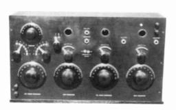
GREBE - Model CR-6 (early), it was the first in the line of the "CR" series. Introduced in the later part of 1919, the CR-6 was a short wave regenerative receiver and two-stage amplifier. Frequency range of the unit was 150-375 and 280-680 meters. The CR-6 was manufactured in both early and late versions. (Craig Huseboe - Marshalltown, IA)
