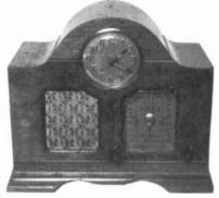
**DETROLA CLOCK RADIO** - Model 3281. Appears in Rider's, Volume 12. Unusual three audio stages with second-stage tube direct coupled to output tube. (George E. Hausske, Wheaton, IL)
