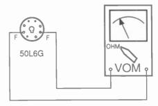
Figure 2. Circuit to check tube filament continuity.
