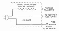
Figure 1. Typical resistance line cord.
