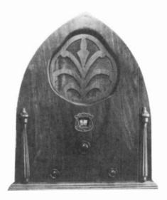
ZANEY-GILL "MUSIC BOX" MODEL 2445 - A six-tube TRF set introduced in late 1930. Believed to have been manufactured by Electrical Research Laboratories, Inc. (ERLA) of Chicago, for the Zaney-Gill Corp. of Chicago and Los Angeles, a pioneer manufacturer of midget radios. (Frank Heathcote, Logansport, IN)
