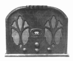
STEWART-WARNER MODEL R-110-AT-Manufactured by the Stewart-Warner Corp. of Chicago. A ten-tube dual wave superhet covering 75-550 meters, it sold for \$49.50 in 1933. Among its features are two 4-inch speakers, automatic noise suppression, push-pull resistance, coupled output tubes, and AVC. (Frank Heathcote, Logansport, IN)
