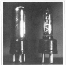
FOR SALE: WD-11 Replacements: N.O.S. Western Electric 215-A tubes mounted on WD-11 bases. Filament 1.1 volts, .25 amps same as WD-11, same vintage, note tip at top, each tube tested before shipment – \$15 each. Can do same for WD-12, WX-12 on your dud base. Also for UV-199, but use only 1 1/2 volts on filament. WANTED: Radiola VI. Accessory items for RA/ DA: DB crystal det., AR RF amp. RT antenna coupler. Charlie Rhodes, Journey's End Rd., South Salem, NY 10590. (914) 533-2503
