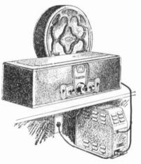
MODEL 601 BANDBOX - The first all metal cabinet radio offered by Crosley was this six tube Model 601 "Bandbox". It was battery operated and outputted to a metal cased dynamic power speaker called a "Dynacone -E". Its price was \$55 without tubes and the speaker sold for \$25. The "Bandbox" featured a licensed Neutrodyne circuit, a first for Crosley in 1928. A 7-tube version (Model 602) was also available.
