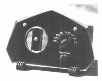
Figure 6. Sparton Model 409-GL with its seven-sided mirrored front.
