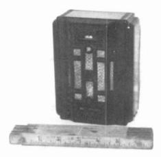
KADETTE - Two tube pocket portable radio, uses #30 tubes and compression type tuning condensers. Has battery plug in rear for 4-prong supply. (Walter Worth - Wollaston, MA)
