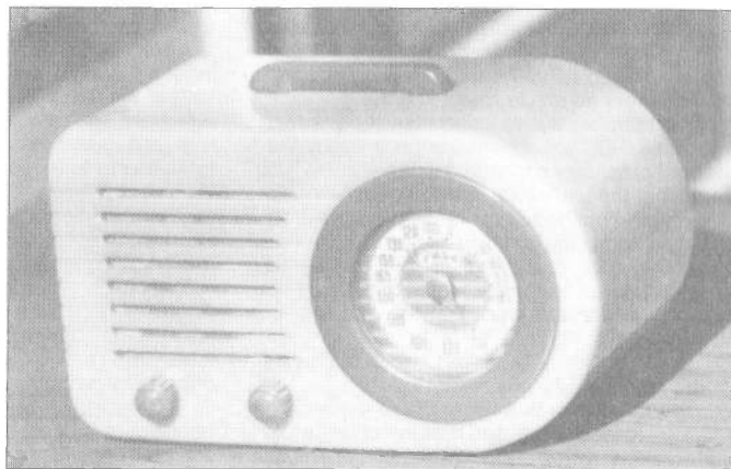
Figure 1. FADA Model 1000 "Bullet" with speaker grille formed as part of the cabinet.
