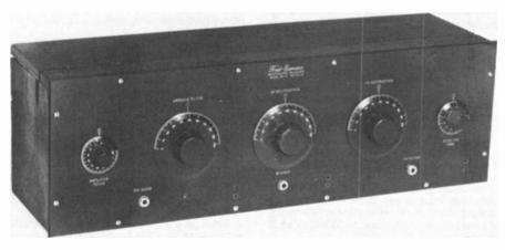
Figure 2. Freed-Eisemann NR-5 radio receiver. The set was advertised as "squealless"; no shrieks and whistles; no longer would choruses of chirping birdies pipe in during the opera or emerge during the Sunday sermon. The "neutrodyne" cir-
