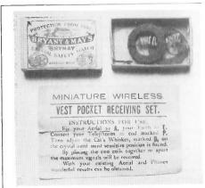
VEST POCKET RECEIVING SET - made by Radiax Ltd., 4 Percy Street, London, 1923. A simple miniature crystal set built into a Bryant & May's matchbox. Primative loose-coupled circuit consisting of two cotton covered wires (the end of one forming the cat's whisker), a piece of brass strip, galena crystal and boot eyelets for Antenna, Earth, and Phones. Size is 3/4 x 21/4 x 11/2 inches. Original price: 2s.6d. (Photo courtesy Jonathan Hill, England.)
