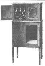
ACE MODEL 3C - The 1924 "Ace"-type 3C was actually the Model 3B redesigned in a square format to fit a large table cabinet like the Crosley Model XL. The two silk-interlined doors opened to expose the radio panel at the left, and included loudspeaker unit on the right. Its price was \$125 without batteries or tubes.
