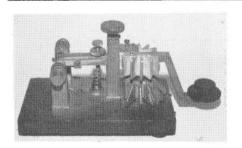
AMERICAN MARCONI - This finned spark key was made in 1917 by the American Marconi Co. for the War Department Signal Corps. It is rated at 50 amps at 250 volts. It is second only in size to the huge Massie Wireless Telegraph Co. keys of that era. A good example of keys used with the "rock crusher" coastal stations then in use. Courtesy R. Rees,
