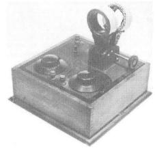
MAGNUM CRYSTAL SET - by Burne-Jones & Co. Ltd., 1930. Crystal set designed for blind listeners. Headphone use only, spring-loaded cat's whisk-er/galena detector, loose-coupled plug-in coils, variable condenser, braille calibrated tuning controls, black Bakelite control panel and knobs, mahogany base 3 x 9 x 9 inches. Donated through the "British Wireless For The Blind Fund." (Photo courtesy of Jonathan Hill, England.)
