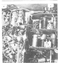
Two multi-section bypass capacitors (upper left) in the Philco 38-3 chassis. The mounting bolts also serve to ground one side of each capacitor. Note the rewound R.F. coils at center right. (Photo by Lance Funderburk)
