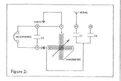
Rotating inductance tuning was used by a number of manufacturers. The Western Electric 44001 (like the W.E. Aeriola Junior in the States), produced in 1922, used the variometer (see Fig. 2 for schematic). Examples of other sets to use the variometer are the "Bijou" by British Thomson-Houston, the Gecophone No. 1 by General Electric Co., and the Walmore Set.
