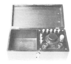
CONNECTICUT TELEPHONE & TELEGRAPH - One tube Sodion receiver, uses nonregenerative Sodion tube. Nice set but very poor sensitivity and volume. Made approximately 1923/24. (Paul Thompson - Santa Barbara, CA)
