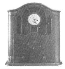
**BULOVA** - This clock radio, model M-701, was made in 1931. Uses 3-51's, 1-24, 1-27, 1-47, and 1-80 tubes. *(Karl Rommel - Lansing, MI)*
