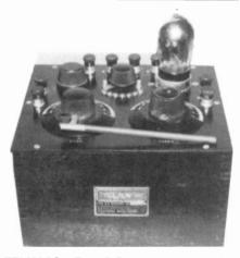
**TELMACO** - Type B-R, a one tube receiver manufactured by Tri-City Radio Electric Supply Co. for the Radio Division Telephone Maintenance Co. This set was advertised in Radio News magazine, May 1923. Notice the "fine tuning stick" attached to dial. (David Mckenzie - Eustis, FL)
