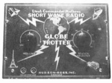
**HUDSON-ROSS INC.** - Called the "Globe Trotter", this shortwave radio uses one 6F7 tube and has a plug-in coil. Made in Chicago, Illinois. (Greg Farmer - Minneapolis, MN)
