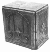
EMERSON - 1933 4-tube radio, model number unknown. Has resistance line cord. Pressed wood panels are tacked to wood frame. Seems to be the same chassis as Mickey Mouse set. (Robert Lozier, Monroe, NC)
