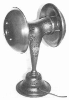
BEST PAL - A most unusual speaker, little is known about this particular model. The label says "Best Pal Loud Speaker" and pictures a horse in the oval decal. The two bowls on each side are made of wood and are used to reflect the sound from the cast iron sound chamber. The speaker stands 16½ inches high. Most likely made by the Pal Radio Co. of Jersey City, New Jersey. Anyone have one in their collection? (Gary Schneider - Cleveland, OH)
