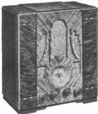
SHORT WAVE and BROADCAST—Model 145 —5 tubes—6 tuned circuits—3 tuning bands include foreign short-wave broadcasting, all American broadcasting, and police, amateur, airplane frequencies. Airplane-type dial is illuminated so that only the tuning band in use is lighted. $59.90 f.a.b. factory.
