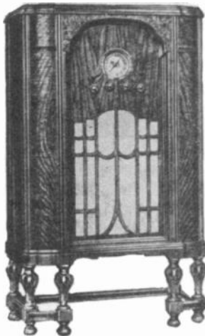
ALL WAVE—Model 318K —8-tube superheterodyne with 9 tuned circuits—complete world-wide range from 540 kilocycles to 22.5 megacycles—in 4 separate tuning bands—2-speed tuning, approximately 6 to 1 and 60 to 1 ratios—shadow tuning—six watts output—11-inch electro-dynamic speaker. Beautiful lowboy cabinet of choice veneers and matched woods with excellent acoustical properties. $89.90 f.a.b. factory.
