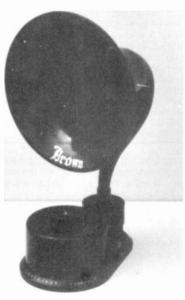
E.G. BROWN CO. - This Brown's Crystavox horn speaker has a built in carbon granule "amplifier", just connect up a battery and you can listen to your crystal set. Made by S.G. Brown Co. in England, circa 1925. (Alan Brehaut - Timaru, New Zealand)
