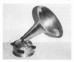
MOON - Unusual speaker manufactured by the Wilson Utensil Co. of Dayton, Ohio. Made of aluminum, it is 15 inches tall and has a bell diameter of 10 inches. Headphones were placed on the two projections sticking out of the base and were used as the driver. (Rudy Burick - Parma, OH)
