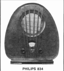
As the radio was not in tip-top shape electrically, I couldn't make an accurate comparison with a comparable TRF to see if the Superinductance circuit was any better. Listening to my local station, there doesn't seem to be much difference. Selectivity was no better than the usual TRF. On more distant stations, the Philips curcuit did seem better compared to a Zenith Model L five tube TRF.
