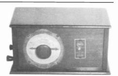
SUPER-BOOSTER- Manufactured by the Liberty Radio Corp. of Cleveland, Ohio and L.A. California, this booster does not contain any amplifier circuit or tubes. It is most likely just a wave trap as the circuit consist of nothing more than a coil and variable capacitor. Nicely constructed in a 9 x 5 x 4½ inch wooden cabinet. (Gary Schneider - Cleveland, OH)
