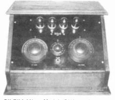
GILFILLAN - Model GN3, a four-tube Neutrodyne featuring exposed tubes on a sloping front panel. (R.A. Hostler - Findlay, OH)
