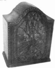
WHAT IS IT? - This set features a Repwood front and solid wood sides. Uses the following tubes: Three 24's, one 27, one 45 and an 80 rectifier. The 24's are highly shielded. This broadcast band set was probably made in the early 30's. Looks as if there was some kind of decal on the inside of the cabinet at some time. Anyone have knowledge of this radio? (Andrew Mooradain, 5 Priscilla Lane, Winchester, MA 01890)
