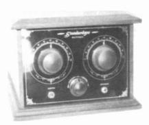
STANDARDYNE - A very unique set using a "multivalve" tube (three tubes in one glass envelope), it was made in 1925 by the Standard Radio Corp. of Worcester, Mass. The sloping front panel is housed in a nice walnut cabinet, measuring 11¾ inches wide, 9 inches deep at base, and 8 inches high. A very desirable set with collectors, this radio is quite scarce, and needless to say, the vacuum tube is almost as difficult to find as the radio itself. (Gary Schneider - Cleveland, OH)
