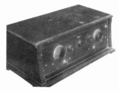
NEWPORT TYPE 1112 - The more expensive Trirduns were housed in more elaborate cabinets like this Type 1112 Trirdyn Special "Newport" that sold for just over \$100. The later Trirdyns panels were slightly redesigned to have the three center knobs align (both rheostats were raised) and the on/off switch moved to the left. Other Trirdyn models had names like "Standard", "Regular", "Biltmore" and "Super".
