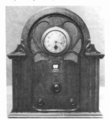
RADA CHRON: Model K-10, a nine tube superhet, manufactured by the Fred Stein Radio Corp., Atchison, Kansas in 1931. - Frank Heathcote
