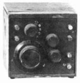
MODEL SR-2 - The smallest Crosley regenerative receiver in a wood cabinet was this "SR-2" one-tube set. It was sold thru Sears and Roebuck exclusively and in actuallity was the Model 50 squeezed so compactly that the panel of the Model 50 had to be rearranged. It was offered to the public for \$23.25 and aimed at the youth market.
