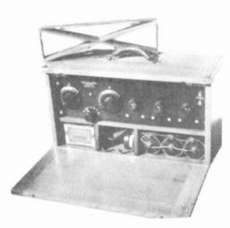
MODEL VIII-P - The Model VIII was sold in a handsome oak portable case that held batteries and phones and antenna wire holder. It's price without the extras was \$60. Adapters were needed to use dry-cell tubes in the porcelain sockets. It's sister set the Model VI (six) also came in an oak portable case for \$40.
