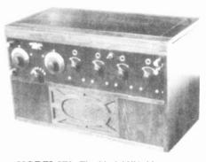
MODEL XV - The Model XV (fifteen) was in reality the Model X in a deluxe cabinet that contained a speaker chamber with a wood horn (no driver) and space for batteries. Access to the set was from the top lid and door panel in the rear. In 1923 it sold for \$70 without tubes, batteries, or antenna. Complete cost was \$127. A similar, but slightly smaller cabinet was sold to house the Crosley VI (six) and was called the Model XII. It sold for \$5 less.
