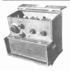
MODEL 52-P - Like the 51, the Model 52 three-tube receiver was marketed in a portable version. The black leatherette case was slightly larger than the 51-portable, but similar in design. Not many of this model seem to exist. Noticeable is the absence of panel binding posts, for they are moved inside to a bakelite strip behind the tube sockets.
