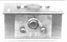
MODEL SR4 - In 1925, Crosley made this onetube portable exclusively for Sears. It was called the SR-4. Captured screws on top released the hinged lid to reveal an ultra-simple circuit using Crosley's latest variable-plate tuning condenser, black molded socket and rheostat. The leatherette covered case would hold the dry-cell batteries and phones. Phone pin holes were panel-mounted. A deluxe version used a brass-plated vernier tuning dial.
