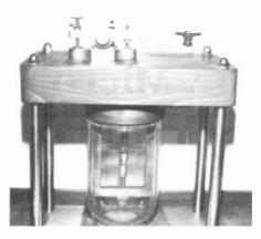
OIL SPARK KEY - This is a Massie Wireless Key of 1904. The contacts were immersed in castor oil to eliminate sparking at the key points. The glass jar was located underneath the table top and only the key mechanism was visible on top. This "one of a kind" belonged to Erwin Rasmussen and later was part of the Guy Martin collection in California. Courtesy Roger Rees.
