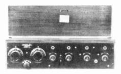
MODEL XJ-Crosley's Model XJ was a later improvement of the Model X and appeared in 1924 at a price of \$65. Inside were the two new molded hard-rubber book condensers, four black molded tube sockets, and a flat, fixed spiderweb coil to replace the older cylinder type. All binding posts were moved inside. A phone jack and a filament control switch were added to the front panel.
