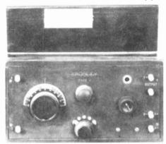
MODEL V-The only difference between the late version "Ace" V and this Crosley Model V...is the name "Crosley" on the panel. The paper tag on the lid made no mention of "Ace" or "Precision". (Some arrangement must have been worked out over the Armstrong patent laws.) This set, somewhat condensed, would reappear later as Crosley's Model 50.
