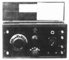
ACE MODEL V-This is the later version of Crosley's "Ace" regenerative Model V. One tube, two less taps on the coil, newer convex styled knobs for the tap switch and regeneration coil which was the new flat spiderweb type. Black molded material replaced the porcelain tube socket and wood book condenser plates.
