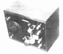
MODEL 1 - The Crosley Model 1 (one) was a completely renewed version of Crosley's first receiver, the tiny Harko Crystal Set. The new box and post matched-up with the Audion Detector, RFTA and 2-Step Audio Frequency Amplifier. Unlike the Harko, its detector was the Wireless Specialty "Tombstone" type. In 1923, it came complete with antenna wire, Crosley brand phones and insulators... all for \$25.
