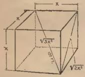
The diagonal of the cube will be the diameter of the sphere, which is 120 feet. Working by the square of the hyptheneuse we get for the value of the diagonal of a side of the cube  $\sqrt{2X^2}$ and for the diagonal of the cube  $\sqrt{3}X^2$ . As this diagonal is 120 feet, we have the equation— $\sqrt{3}X^2 = 120$
