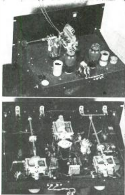
Top and bottom views of the exciter chassis. The T-40 shown replaces the original T-20. Note Ward Leonard keying relay mounted between the 6L6 tubes. Neutralizing condenser. Cy. has a bakelite extension shaft.
