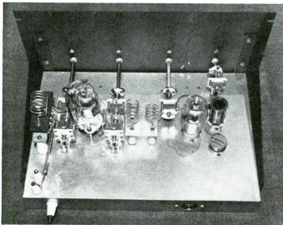
Chassis view of the complete r.f. section showing details of coil mountings and relation of components.
