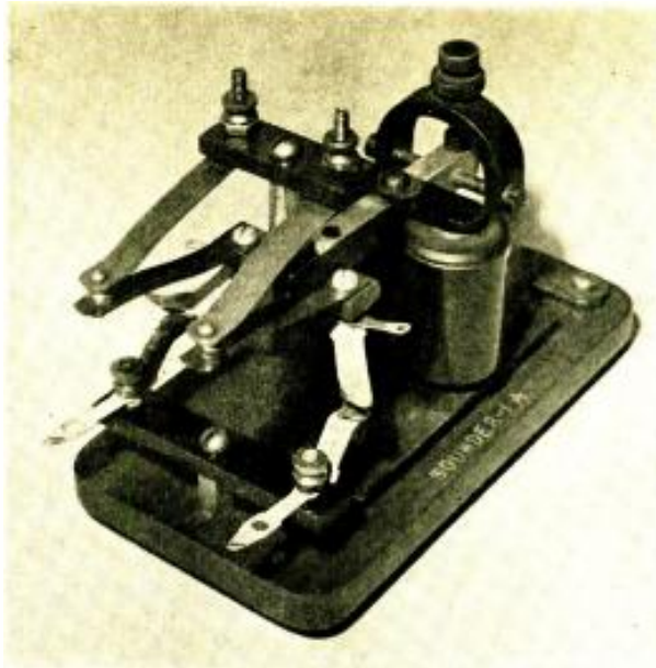
Automatic antenna switching relay made from a Bunnell Telegraph Sounder.
