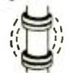
Bottom—No shield between coils in ordinary radio. Signals jump back and forth, making howl. Factory cuts sensitivity to end howl—thus you miss many stations.
