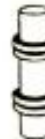
Bottom—2 section coils of ordinary radio. Mounted vertically. Wood dowel shrinks in dry climate—coils slip down. Expands in wet climate—compresses wires, causes short circuit.
