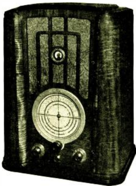
Fig. 1. The Pilot Model 293 All-Wave Receiver with electron-ray tuning indicator.
