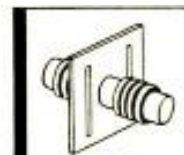
Top—SCOTT brass shield between primary and secondary coils. Increases sensitivity which can be built into set. Enables you to get more stations.
