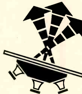
Unique "wide-angle" concave tweeter array — cuts through on-stage volume, eliminates "beaming" on-axis and muddy sound off-axis.
