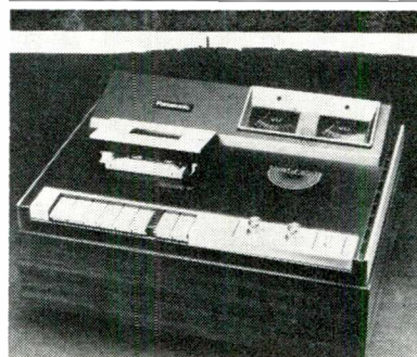
The Panasonic Color Picture Cassette Player: note audio cassette half-way into slot as in standard audio cassette player units.
