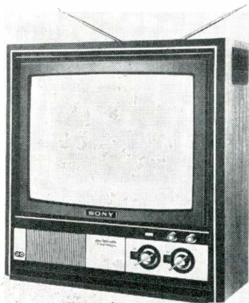
Sony's KV-1722 Trinitron tv, one of their new short tube color tv's.
