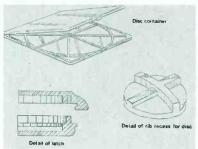
The new package has sturdy rib supports that prevent inserted disks from rubbing, bending or shifting about in their containers. Made of polypropylene, and mass-produced by plastic mold insertion, they add a 3-dimensional graphics capability to record packaging. Schidlowski also points out that, "outer cardboard crating becomes completely unnecessary since Disq-Paks can be mailed directly after they are shrink wrapped."
