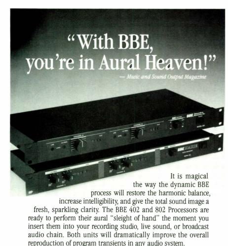
The BBE processors achieve *time-alignment* of harmonic and fundamental frequencies that were present in the live performance but became re-shuffled in the often convoluted paths of recording, playback, and broadcast of audio.
