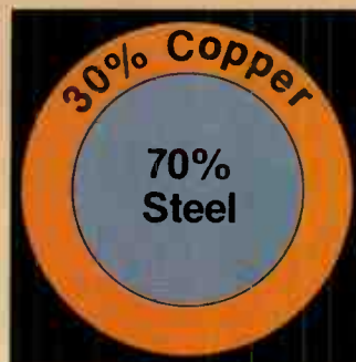
Cross section of XL Reds' copper coated steel wrap (winding) wire.
