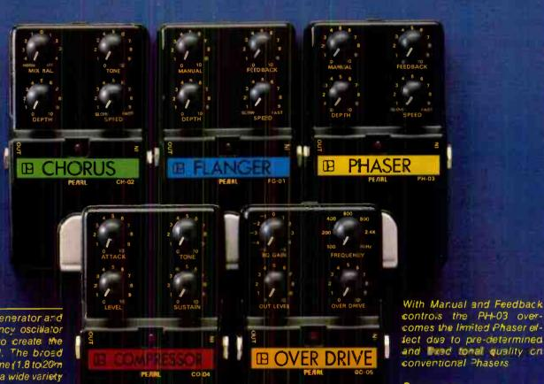
A clock pulse generator and ultra-low frequency oscillator are combined to create the flanging sound. The broad range of delay time (1.8 to 20m seconds) makes a wide variety of sound effects possible: medium delay gives orthodox flanger and chorus effects: shorter delay sounds more like phasing; dual voice and metallic reverberation effects are created with a long delay.
