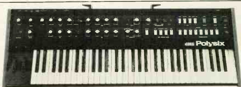
Korg Polysix synthesizer: 6 voices, 32 programs and built-in arpeggiator for under $2000.
