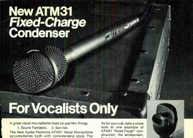
sound is the direct result of new condenser technology from A-T. Our unique fixed-charge condenser element puts the electrical charge on the back plate rather than on the moving diaphragm. So the diaphragm can be made thinner, better able to react precisely to every vocal nuance.
