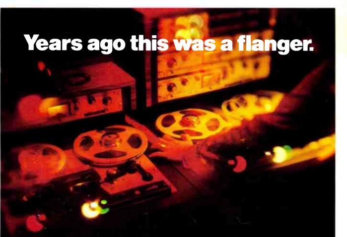
Incredible, isn't it? But when flanging was first used, it was done like this. Rumor has it that the first time flanging was achieved, it happened by accident. An engineer mistakenly leaned on the flange of a moving reel altering its speed relative to another simultaneously moving machine. The sweeping sound that resulted was one of an enhanced tonality, similar to a phase shift but also having characteristics of its own. This phenomenon because the better new sound in the recording indi-
