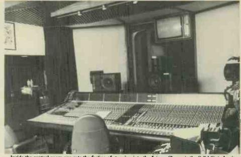
Inside the control room one gets the feeling of stepping into the future. Shown is the Solid State Logic 4000E console with total recall computer and overliead video display monitor.
