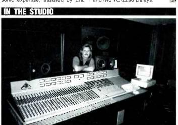
Producer/studio owner Dino Maddalone is pictured with the new MTA Series 980 recording console. Designed by Malcolm Toft in London, this console is a fully computer automated recording/mixing desk, with Uptown moving faders, and was specifically designed and built for Maddalone's Dino M III Recording Facility in Torrance.
