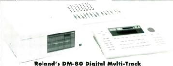
The DM-80 is an eight-track, hard disk based digital audio recorder/editor. As a stand alone unit costing under \$10,000, the DM-80 has features such as: non-destructive editing, random-access recording/playback and complete interfacing capabilities to fit any application in audio recording or video post-production work.
