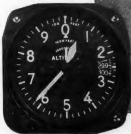
The C-12 altimeter made by Buescher is accurate to within 20 feet from sea level to 50,000 feet, yet it must be rugged enough to take the gun shock of cannon firing, dive strains, and rough take-offs and landings. It must operate perfectly at 150° F above zero and at 70° F below zero. Buescher altimeters are used in every type of Army and Navy plane from the tough, speedy fighters, to the huge precision bombers.
