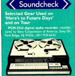
The PCM-3324 is the heart of Sony's multichannel digital recorder series, featuring 16-bit linear quantization capability and a new code format, which together provide an incredible dynamic range of over 90db. Reliable electronic editing and tape-splice editing are possible with the PCM-3324, and the unit is equipped with both analog/ digital and digital/analog converters, along with digita and analog terminals. The 24-channel machine also features a new pinch-rollerless tape transport system.
