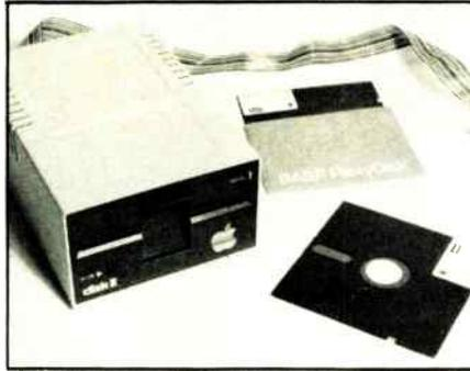
An Apple II disc drive with floppy discs (diskettes). The magnetic disc itself is permanently housed in a protective sleeve (front). When not in the drive, diskettes should be kept in their dust covers (back) otherwise the disc surface may be damaged and files become irretrievable.
