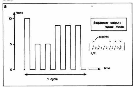
A sequencer-generated repetitive waveform which could be used to superimpose rythmic patterns on audio signals passing through the VCF and/or VCA.
