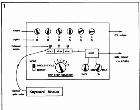
Front panel of a sequencer with six stages. For the production of automatic sequences, an internal clock is included which can be started and stopped either manually (using the push buttons) or by remote control (via the external inputs). With the external connection shown here, the sequencer will start when any key is pressed down.
