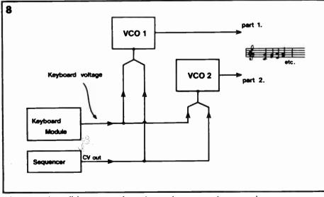
A sequencer's parallel outputs can be used to produce passages in two-part harmony.
