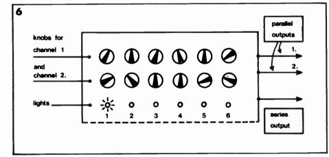
Part of the front panel of a two-channel sequencer. The sequencer has three outputs: two parallel, and one series. Using the parallel outputs, two voltage-controlled modules can be independently controlled at the same time. The series output is used to produce longer sequences, up to 12 steps long in this case.
