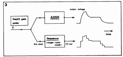
A sequencer can be used in the same way as the ADSR module to generate a particular waveform coincident with each key depression. Note however that although the sequencer cycle starts when the key is depressed due to the external start connection, the sequencer's output (unlike the ADSR waveform) is not dependent on the key release.
