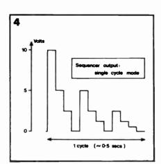
A complex waveform generated by a 12-stage sequencer operating in single-cycle mode which will produce echo effects when used as the control voltage for a VCA.
