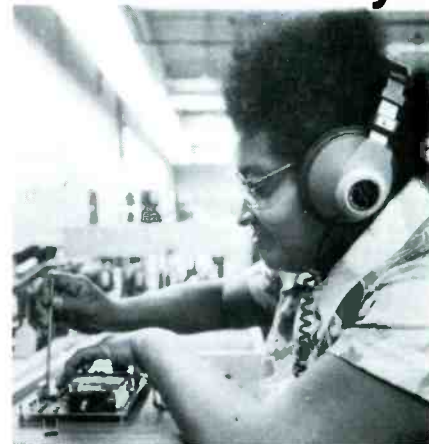
WITH THE ACCENT ON SOUND — This photo, taken at the Williams factory, shows a plant employee utilizing a customized test fixture and a special pair of earphones to make a final check on the factory's noted sounds components.
