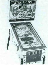
demon outhole. The second new technique consists of two 'ball-saver' bumpers. A ball headed for outhole may hit live rubber bumpers at the bottom of the playfield and bounce back into action area.
