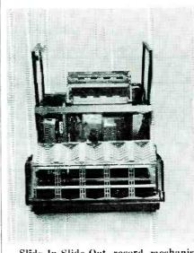
Slide-In-Slide-Out record mechanis is designed to reduce record changing time for the routeman. When doors are opened, the entire mechanism rolls forward for necessary changes. Re-cord changes can be made without "scanning." The entire Gem concept cord has been developed to enhance servic-ing speed and reduce servicing costs, according to the factory.
